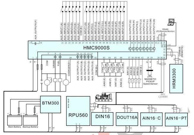
Fig. 5 HMC9000S Typical Wiring Diagram
