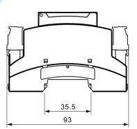
Fig.6 Overall Dimensions (Unit: mm)
